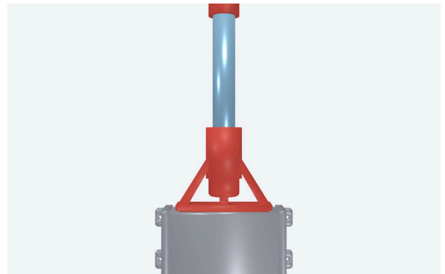
Figure 2: Top view: antenna perpendicular off the enclosure’s ribbed side, centred; dielectric A-frame mount.
